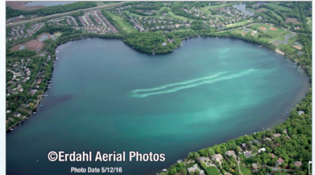
Alum Floc Trails Behind Barge at Lake Riley, 2016
