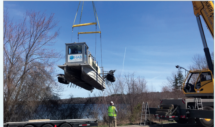
Lowering HAB's Application Barge into Moswansicut Reservoir
